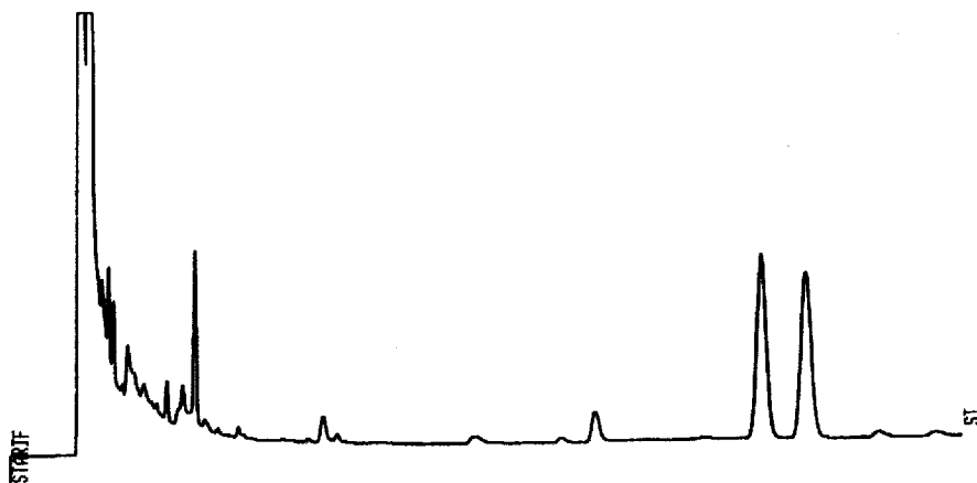
Fig. 4. Gas chromatogram of the mixed derivative in Fig. 3b. Column temperature, 250°C. Retention time for peak 2, 12 min.
